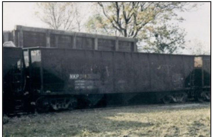
Fig. 5 - This photo is from 1988. Although there is a hopper waiting to be loaded, the construction of the upper part is visible with the 10" x 10" horizontal timber on the top and the metal straps holding it in place.
