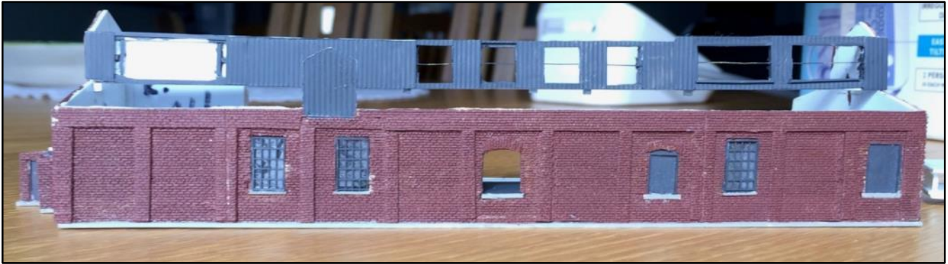
The CSB under construction. The side walls are laser cut brick sheet over .040” styrene sheet backing; the clerestory walls are corrugate styrene siding. You can see the .020” brass wire used to glue the open center-pivot windows.
