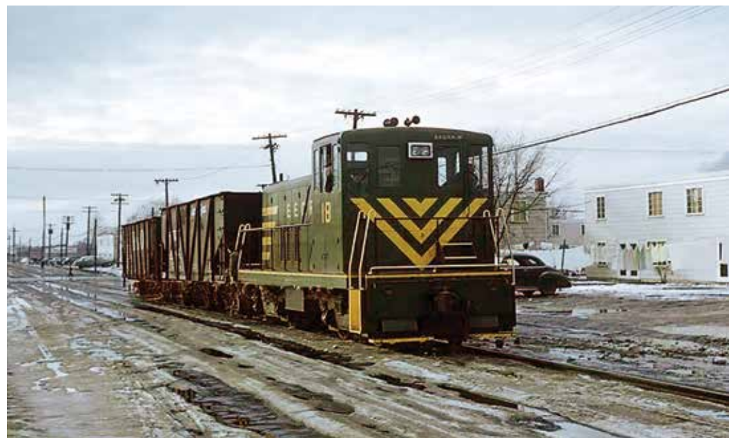
BELOW: The East Erie Commercial Railroad was incorporated in 1907 to serve east-side industrial concerns in Erie, but principally the General Electric Company and later its locomotive-building facility. EEC 70-tonner No. 18—a GE product, of course—shuttles along 10th Street near Tacoma Avenue on PRR trackage.
